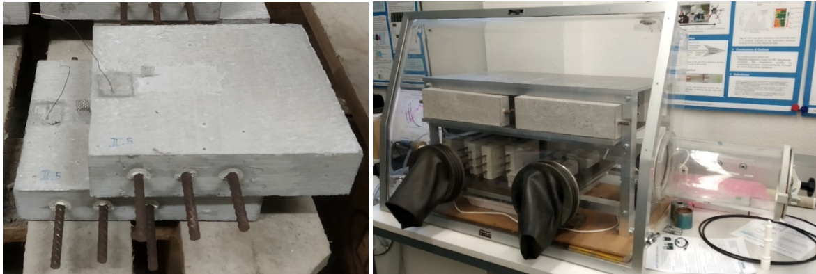
Figure 3 a) Concrete specimens for corrosion rate measurements in Phase 2. b) Carbonation box.
