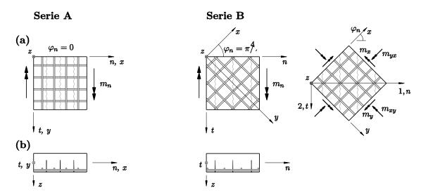
Testing program series A and B: (a) plan views with reinforcement, bending demand and cracking pattern; (b) sections.
