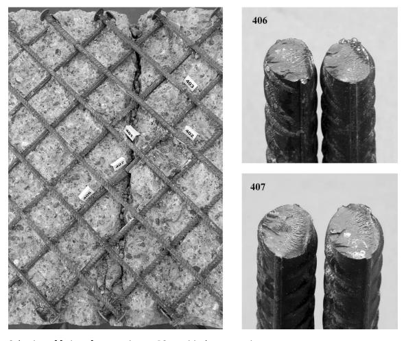
Selection of fatigue fractures in test B2 at critical cross-section.
